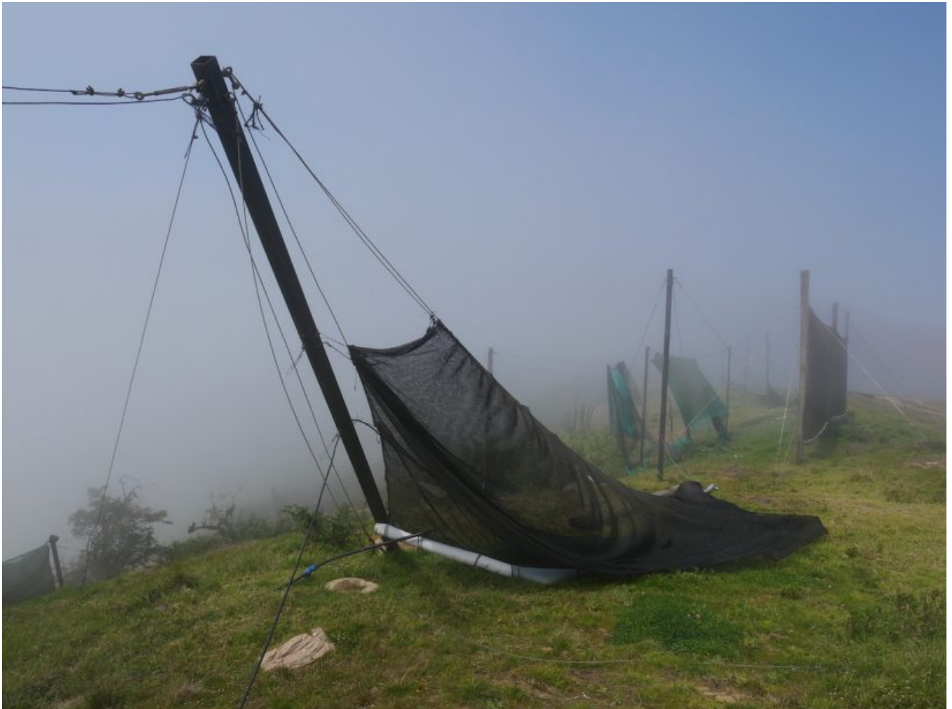
Fallen fog catchers in the Atiquipa fog oasis ecosystem. Photo by the author.
